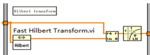
Fig. 7 the Hilbert transform procedure (the input signal is on the left, the output signal is on the right)
