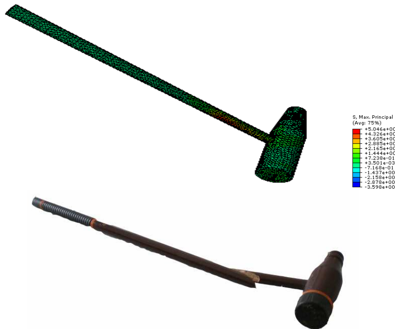
Fig.2 The maximal stress distribution of mallet (top) and fracture mallet in real performing event (bottom)
