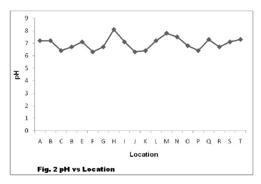
The above graph represents the pH value of the samples analysed of wastewater from various Lagoons and Drains. The pH lies between the standard ranges of 6.5-9 (CPCB). The maximum value is 8.1 of 'Chandaniya' Gandhi Eye Hospital and the minimum value is 6.3 of Mathura pumping station. The average is 6.98 i.e. 7 (approx.).
