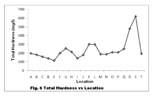
The graph represents the total hardness in terms of mg/l as CaCO<sub>3</sub>. The maximum being of Aligarh drain final output i.e. 620 mg/l and minimum being 141 mg/l of Loco Colony Main. Aligarh drain has such a high concentration as compared to the rest of the samples because it carries industrial wastewater. The average value is 236.6mg/l.
