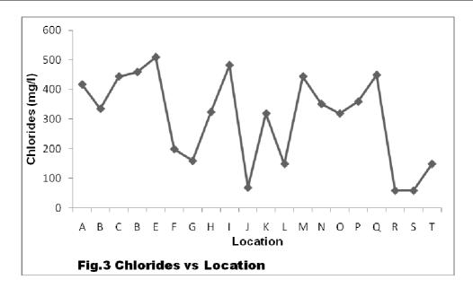
The maximum chloride concentration is 510mg/l of Gular road inlet and minimum is 60 mg/l of the Aligarh drain. The high concentration of Gular road inlet may be a result of point source contamination as the concentration of the lagoon itself is around 200 mg/l The average concentration of all the Lagoons and drain is 312 mg/l. Chloride concentration are within the prescribed limit at all the locations.
