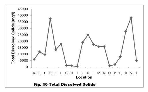
The graph represents the total dissolved solids in mg/l. The maximum value is 38400 mg/l of Aligarh drain final output and the minimum is 300 mg/l of Laal Diggi. The average value is 13660 mg/l.
