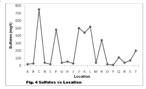
The graph represents the sulphates concentration of the samples of wastewater analysed from different lagoons and drains. The maximum concentration is 750 mg/l of Loco colony inlet the minimum being 10 mg/l of Surendra Nagar lagoon. The average concentration is 311 mg/l.
