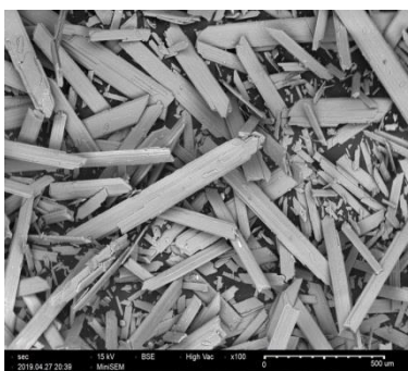
Figure 1. Morphological characterization of phosphogypsum by SEM
