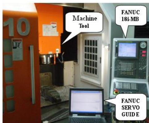
Figure. 4 The actual experimental machine: the H10 high-speed machine tool
