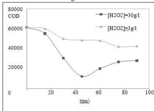
Figure 5: Evolution of COD over time for  $[H_2O_2] = 30$  g/l and 3 g/l
