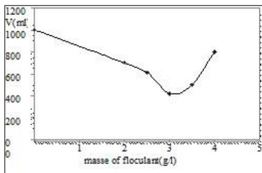
Figure 2: Evolution of settled volume of OMW depending on the mass of flocculant
