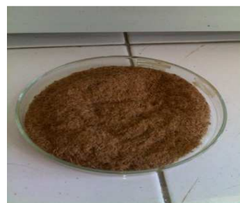
Photo2- crushed Eucalyptus bark after Chemical-treatment
