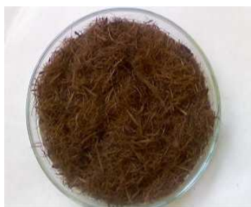
Photo1- crushed Eucalyptus bark before Chemical-treatment
