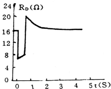
Fig.5 The experimental result of instantaneous change behaviors of electrical resistance of the PC-type  $HgCdTe$  detector irradiated by  $1.06 \mu m$  laser
