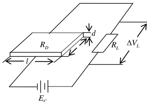
Fig.1 The working principle graph of PC-type detector
