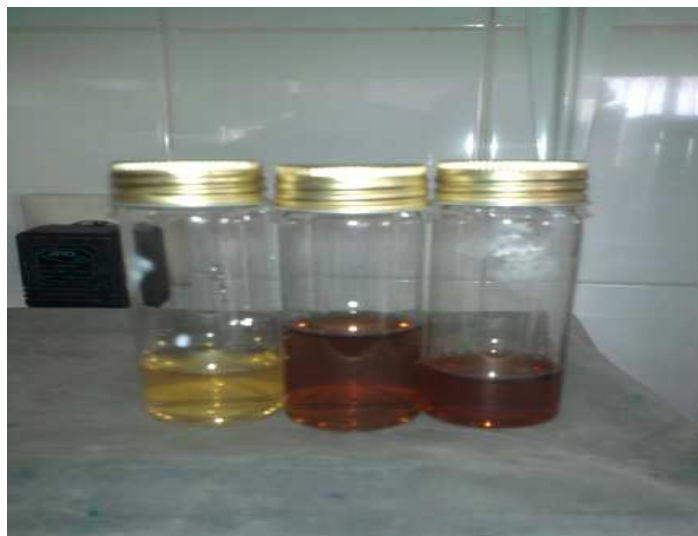
Fig.1. Change of color from pale yellow to dark brown by the addition of silver nitrate
