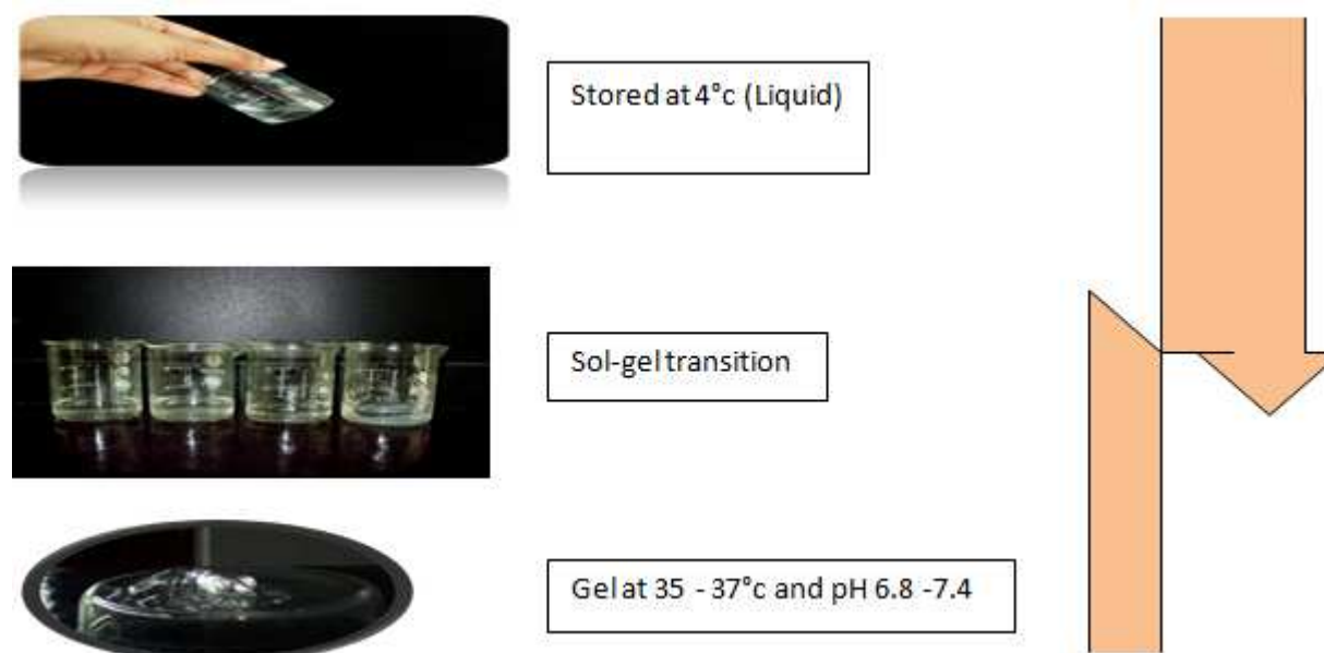
Figure 6: Figure showing the sol to gel transition of in situ gel formulation
