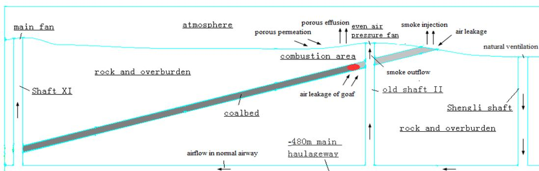
Fig. 3: Simplified graph of the thermal dynamic system in the outcrop fire area of old Shaft II
