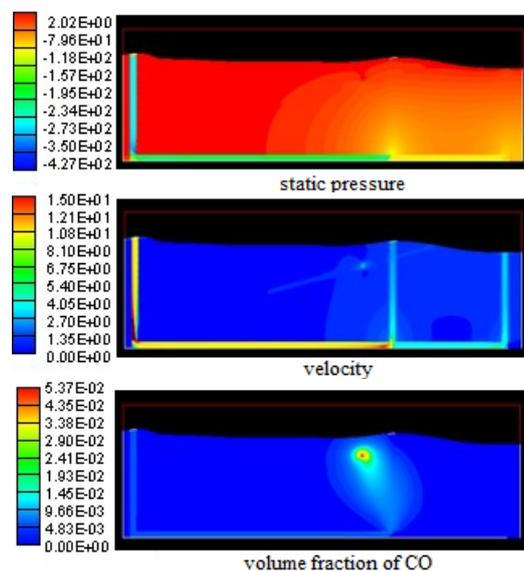
Fig. 6: Pressure field, velocity field and CO concentration field of coal fire after stopping the even pressure fan of old Shaft II
