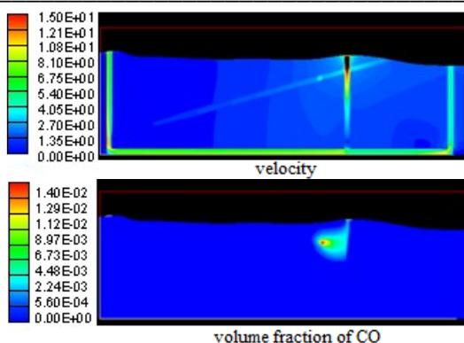
Fig. 5: Static pressure field, temperature field, velocity field and CO concentration field when the fan of old Shaft II starts
