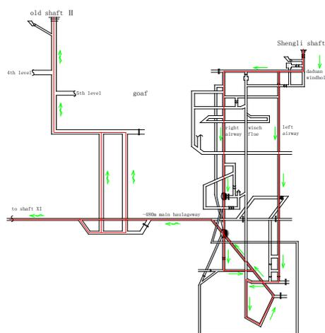
Fig. 2: Ventilation system scheme around the fire area
