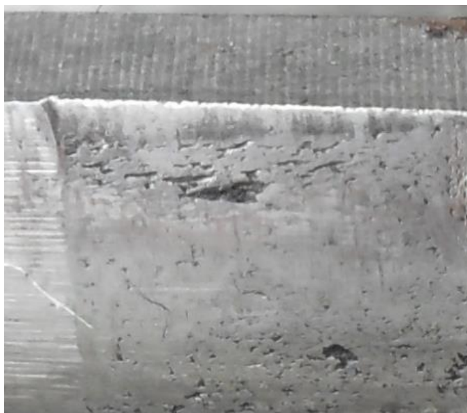
Fig.6 The morphology of gear addendum fatigue crack
