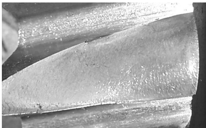
Fig.4 The morphology of test gear fatigue fracture
