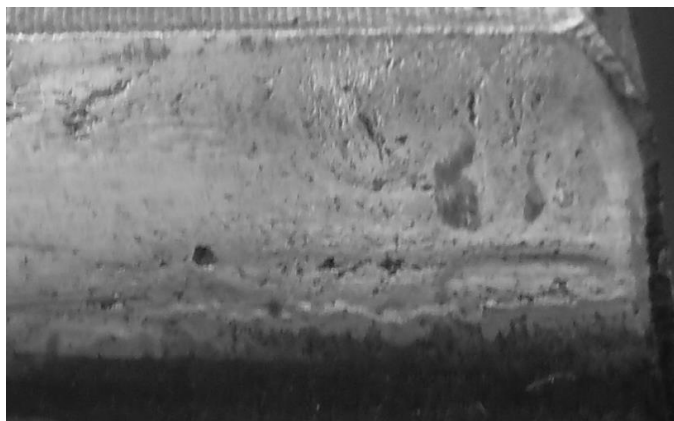
Fig.5 The morphology of gear surface fatigue crack
