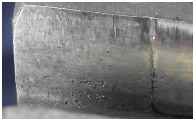
Fig.7 The morphology of surface fatigue during running-in
