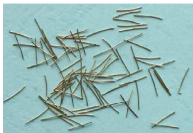
Figure 1. Steel fibers used for SFRC composite
