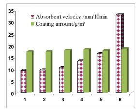
Fig. 5. Coating amount as a function of absorbent velocity of reconstituted tobacco sheets (\*solid content of the tobacco extract was 41.2%, temperature was 22 ° C, coating machine speed was 10m/min, tobacco extract flow was 4.35 ml/s)
