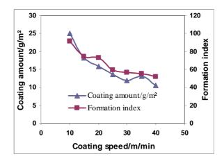
Fig. 3. Coating amount and paper sheet formation as a function of coating speed (\*solid content of the tobacco extract was 41.2%, tobacco extract flow was 3.45ml/s)
