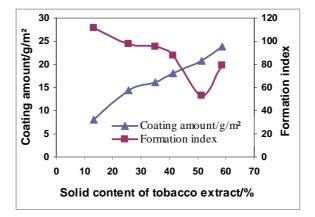
Fig. 1. Coating amount and paper sheet formation index as a function of solid content of tobacco extract(\*coating machine speed was 20 m/min, spraying flow was 3.45 ml/s)
