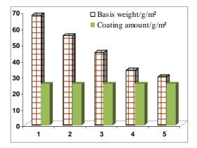
Fig. 4. Coating amount as a function of basis weight of reconstituted tobacco sheets(\*solid content of the tobacco extract was 41.2%, temperature was 22 °C, coating machine speed was 10m/min, tobacco extract flow was 4.35 ml/s)
