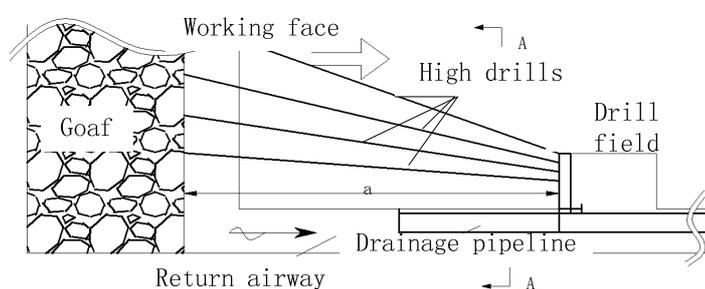
**Fig.1** The plane arrangement of high position drills in working face
