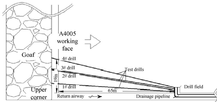
Fig.4 The arrangement of test high drills
