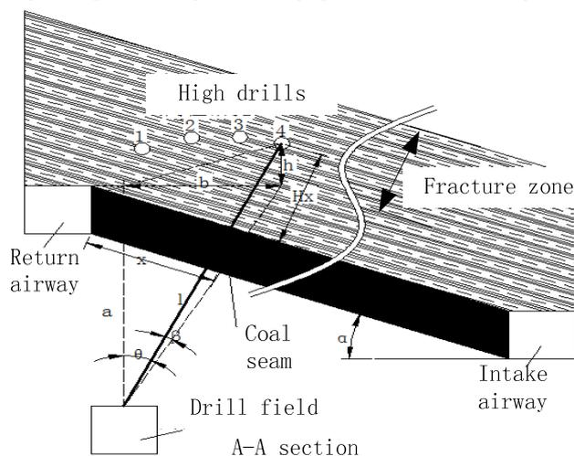
**Fig.2** The sections arrangement of high position drills in working face
