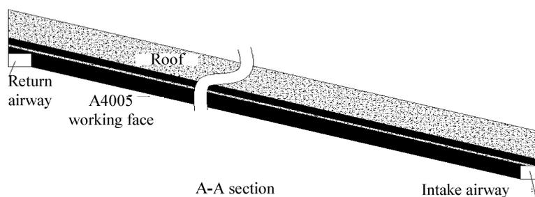
Fig.3 A4005 Working-face arrangement
