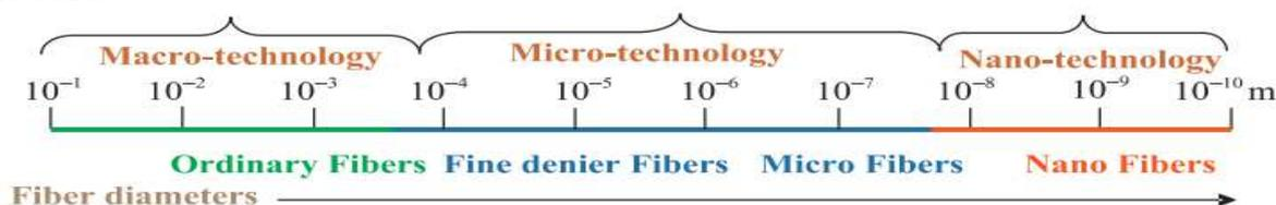
Figure 1 Fiber size and associated manufacturing/processing technologies
