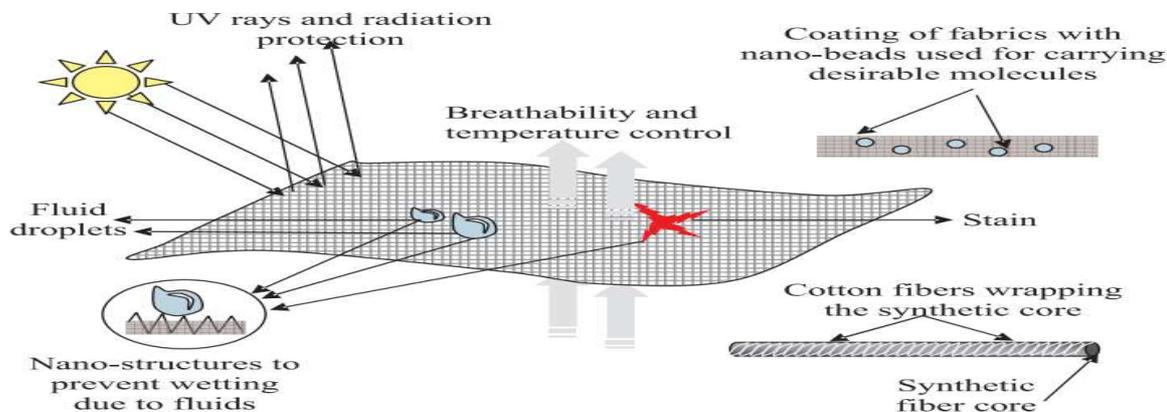
Figure 2 Fabric finishing for enhanced properties and performance
