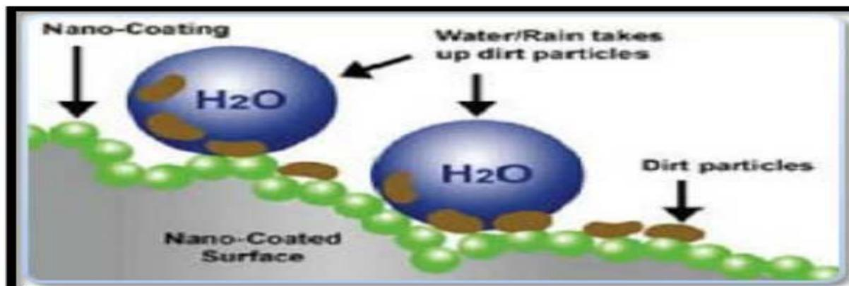
Fig. 3 Nano-coated self cleaning textile
