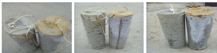
Figure 21 The comparison of concrete between Steel Casing protection and no protection after 300 times freeze-thaw cycle
