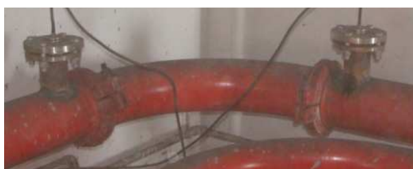
Fig 3 The elbow section used for determination of local resistance loss
