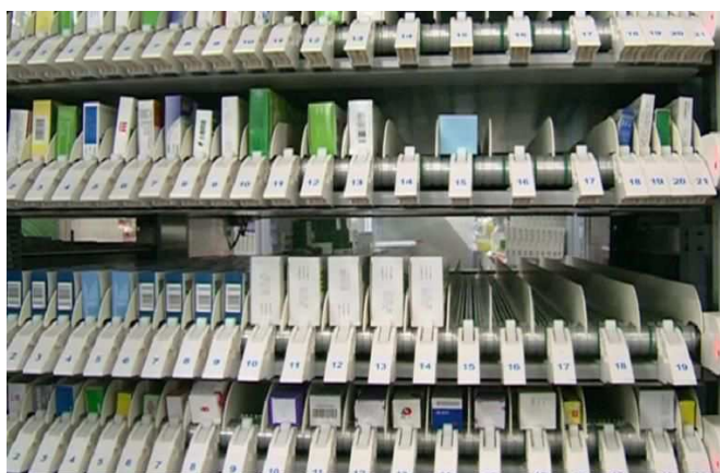
Fig.1 The medicine cabinet of automatic drug delivery machine
