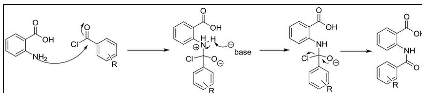
Figure 1: The first mechanism of the reactions
