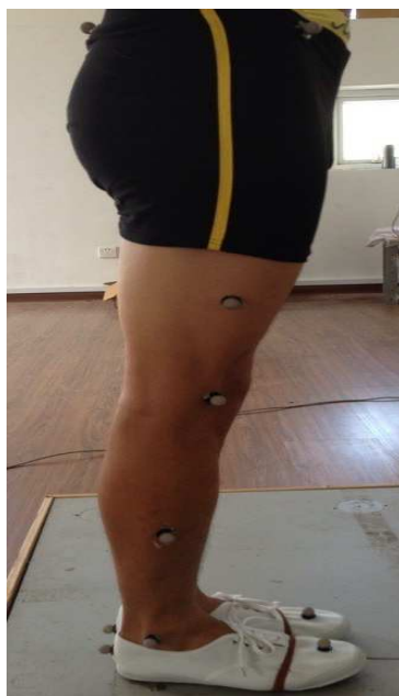
Figure. 1 Reflective markers placed on the one side of the lower limb.
