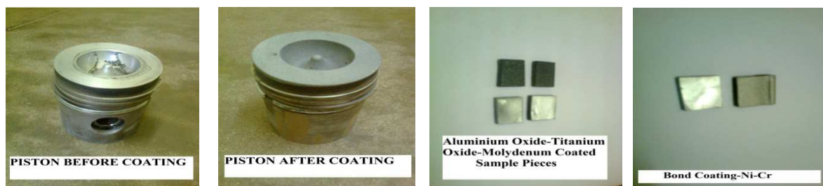
Fig. 1. Piston crown for coated and uncoated and specimens
