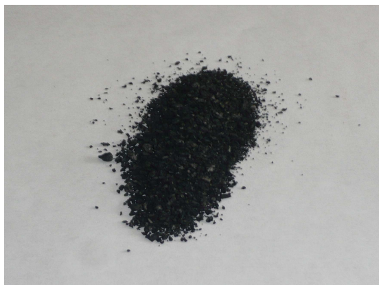
Figure 1. Sorbent from grape seed meal
