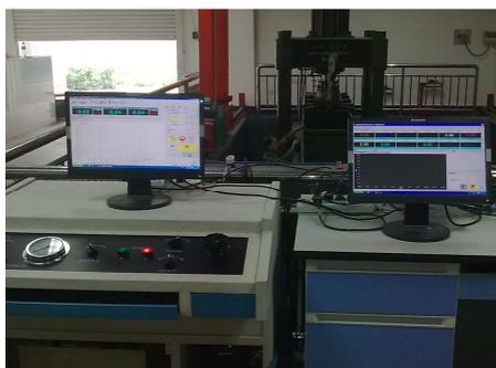
Fig. 1 the microprocessor control electro-hydraulic servo tester's measurement and control system
