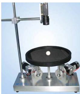
Fig. 1: Ball and plate system
