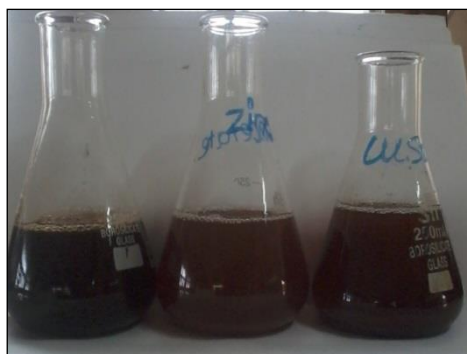
Figure 2: Solution of extract, zinc and copper nanoparticle synthesised after 24 hrs
