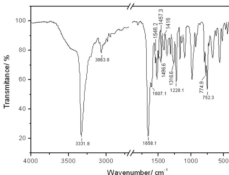
Figure 1 IR spectra of BAH
