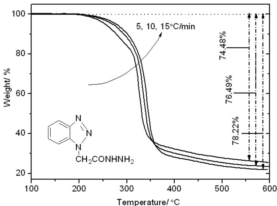
Figure 6 Thermal decomposition of BAH
