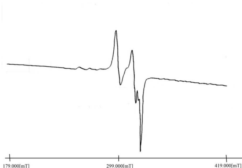
Figure 9. ESR spectrum of [\text{CuL}_2\text{Cl}(\text{H}_2\text{O})]\text{Cl}\cdot\text{H}_2\text{O} complex
