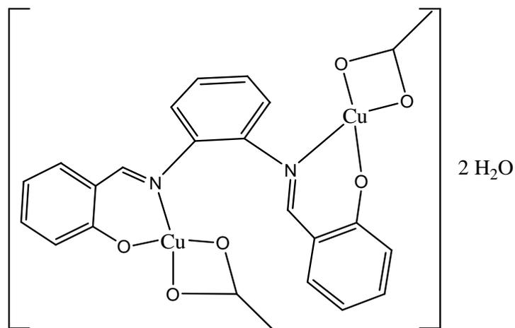
Fig. 5. Suggested structure of Cu(II)-mixed ligand complex (3) containing salen and acetate
