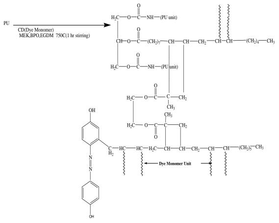
Polymer Blend of Cardanol based dye with 4-aminophenol and Polyurethane of modified Linseed Oil with DPMDI
