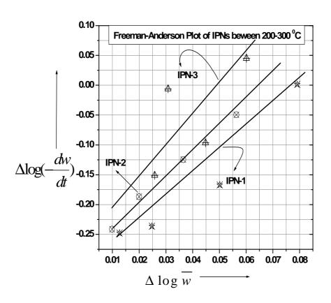
Figure 7: Freeman-Anderson's Plot of the Polymer Blends in the temperature range of 200-300<sup>o</sup>C
