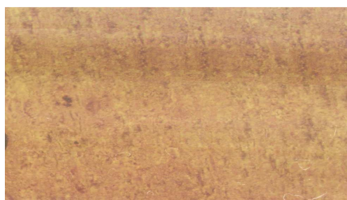
Figure 2. a: Schlieren texture of the smectic (Sc) in heating of L6, b: Marble texture for Nematic phase in heating for L3, C: Schlieren texture for Nematic phase in cooling for L3 .
