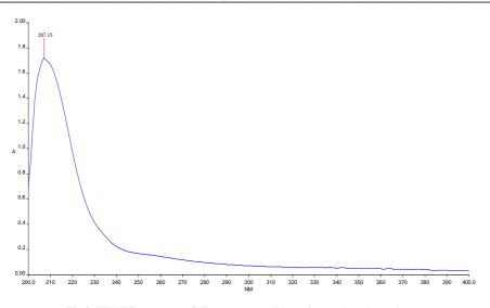
Fig.3. UV-VIS spectrum of silver nano particles using methanol as solvent
