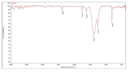
Fig.4. FT-IR spectrum for the silver nanoparticles
