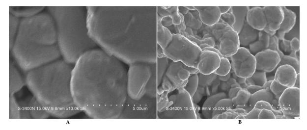
Fig.2. A&B - SEM micrograph of the silver nano particles
