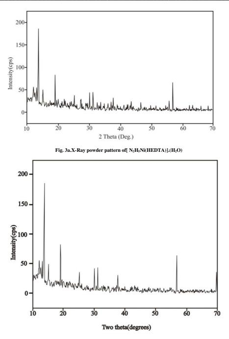
Fig. 3b.X-Ray powder pattern of [N<sub>2</sub>H<sub>5</sub>Co<sub>2/3</sub>Ni<sub>1/3</sub>(HEDTA)].(H<sub>2</sub>O)
