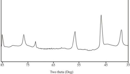
Fig. 5. X-Ray Powder diffraction pattern of NiCo<sub>2</sub>O<sub>4</sub>
