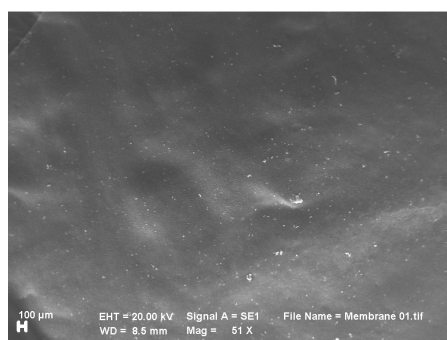
a) The optimum hybrid zeolite A(70%) chitosan sulfonated membrane
