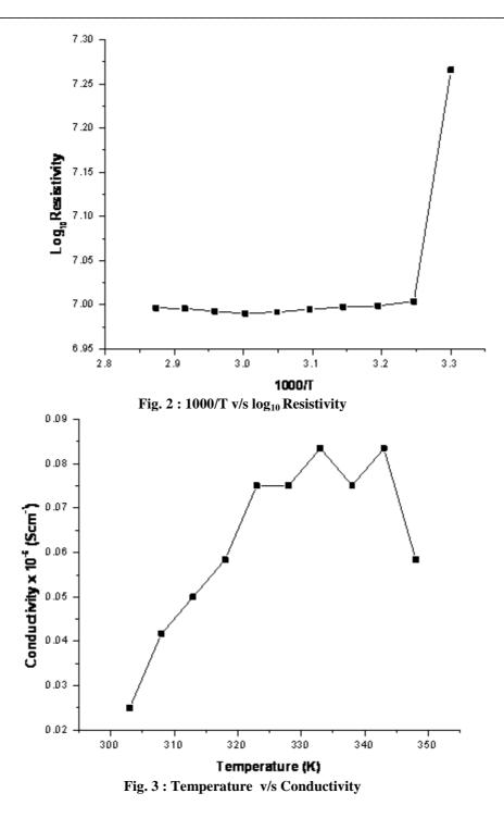
The experimental data of conductivity measurement of  $\alpha$ -naphthol (p-choranil) are given in Table (4). These data are graphically represented in figure 3 (as  $\sigma$  v/s T curves) and figure 4 (log<sub>10</sub>  $\rho$  v/s 1000/T curves).
