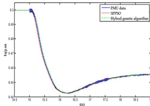
Figure4. Comparison result of simulation data and PUM data of q axis
