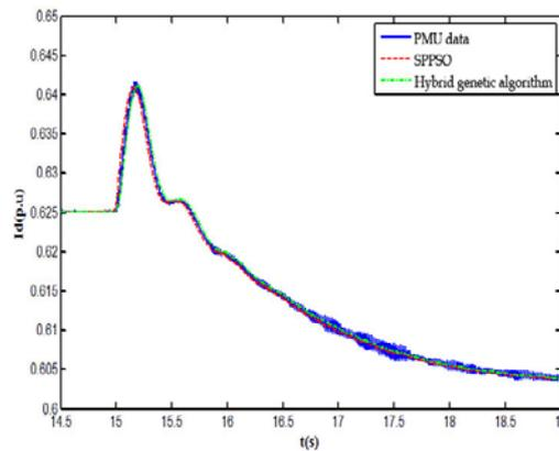
Figure3. Comparison result of simulation data and PUM data of d axis
