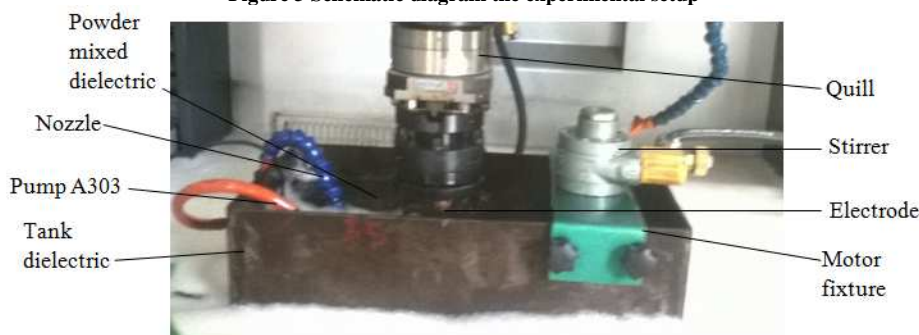
Figure 4 Photograph of the experimental setup
