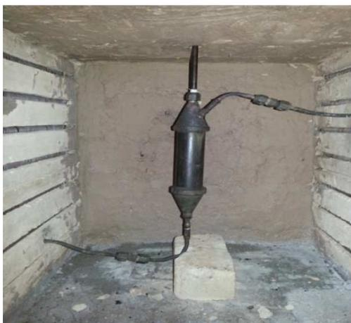
**Photograph 3: Sample holder for burning of sample at elevated temperature**
