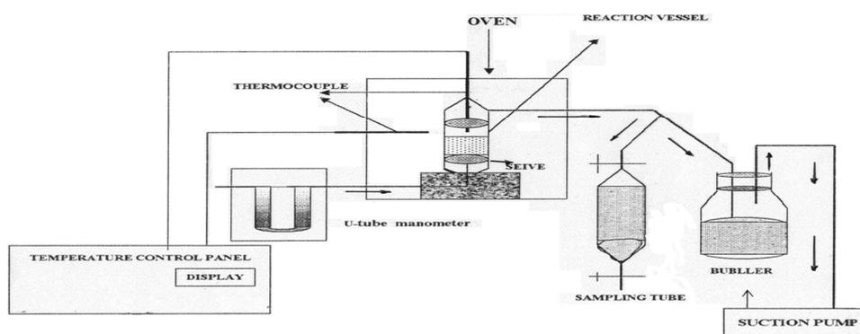
Figure 5: Set up for Thermal decomposition study
