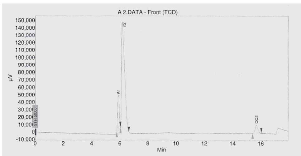
Figure 7: GC graph for Hard Coke + THERMACT-BF
