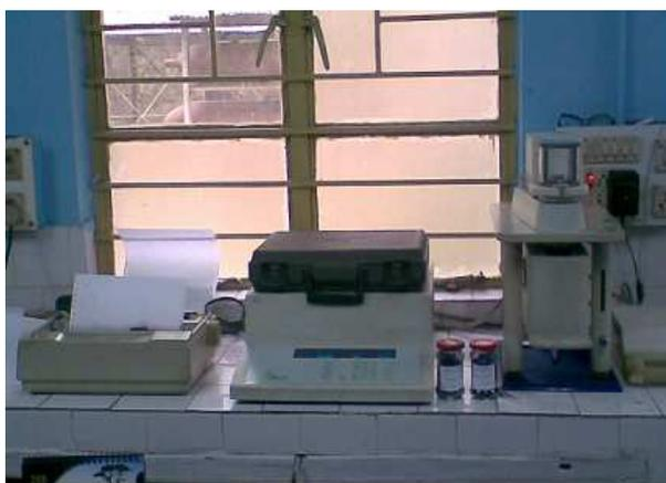
**Photograph 1: Thermo Gravimetric Analyzer (Model TG-50, Mattler)**
