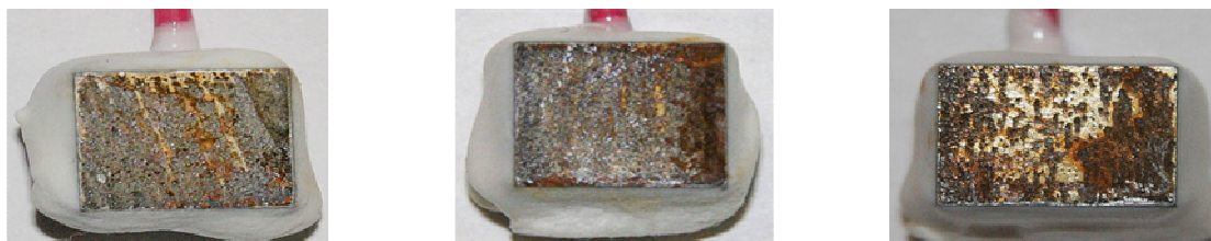
Figure 8. Comparison of three sample coupling surface corrosion
