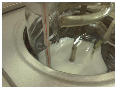
Figure 2 PU/PA emulsion preparation
