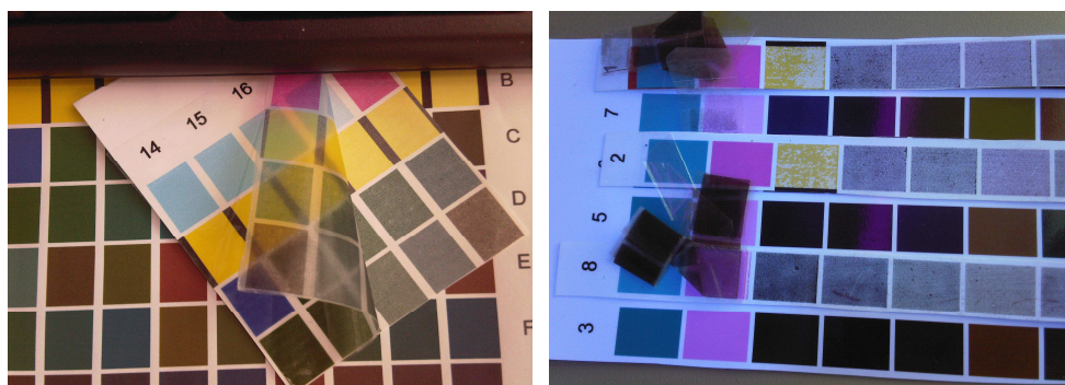
Figure 8 The ink removing on uncoated film and coated film
