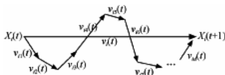
Fig. 3: the process of the particle position update
