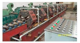
Fig. 1: Y-shaped three-roll mill production line
