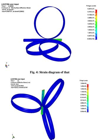
Fig. 5: Stress diagram of rolling bitten into the second pass stress
