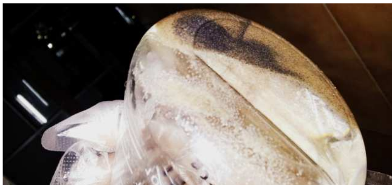
Fig3 – Formation of dark blue precipitate in the acid treated sand
