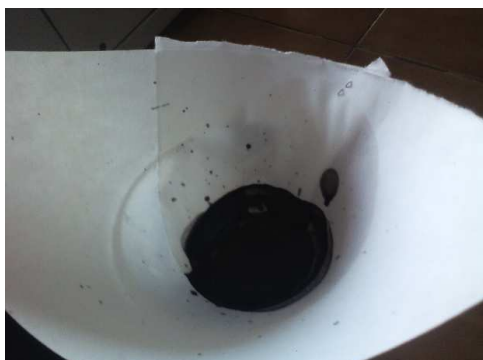
Figure: 3 Separation of iron nanoparticles
