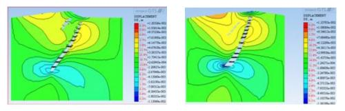
Horizontal displacement echogram to excavated ore of No.1&No.2 exploration line
