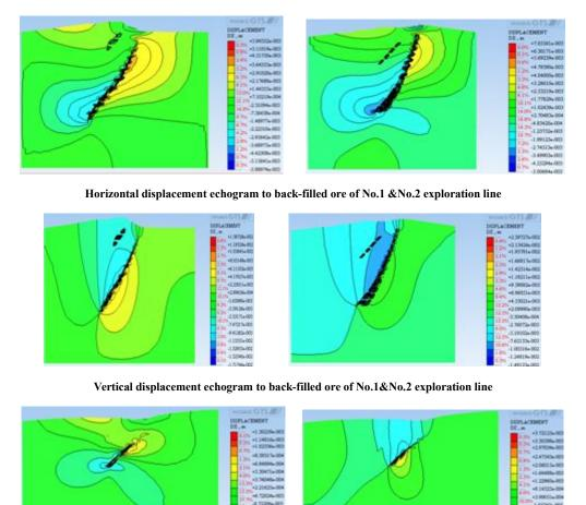
Horizontal &Vertical displacement echogram to back-filled ore of No.5 exploration line
