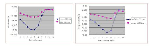
Comparison of displacement changes before filling and after filling to ground spot of No.1 &No.2 exploration line
