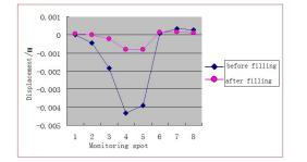
Comparison of displacement changes and after filling to ground spot of No.5 exploration line
