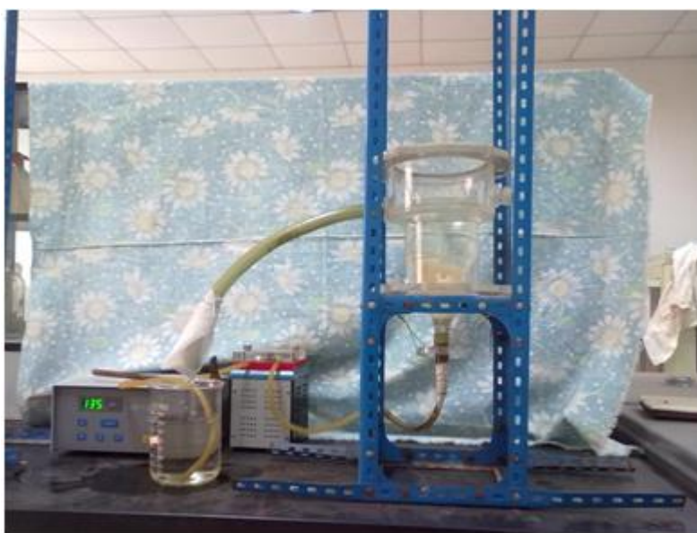
Fig.3-Physical map of the fluidized bed laccase reactor system
