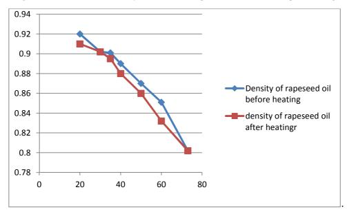
Figure 4: Representing the density variation of rapeseed oil before and after heating
