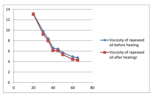
Figure 3: The variation of the viscosity as a function of temperature before and after rapeseed heating
