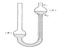
Figure 2 :Ostwald viscometer
