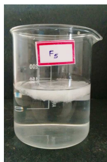
In-situ gel containing 1.5% SA & 0.5% \text{CaCO}_3 (F5)
