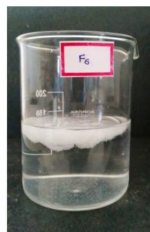
In-situ gel containing 1.5% SA & 0.75% \text{CaCO}_3 (F6)
