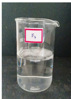
In-situ gel containing 1.5% SA & 1.5% \text{CaCO}_3 (F7)
