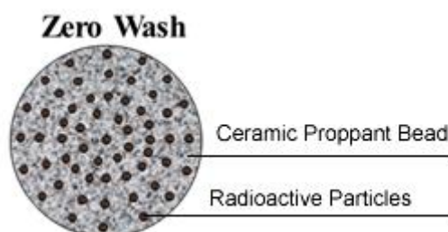
Fig. 1. Zero Wash Coating tracer structure diagram
