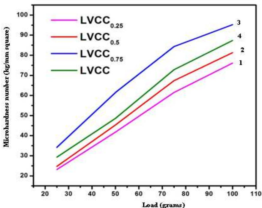
Figure 1: Dependence of hardness on load for various concentration of cadmium chloride mixed LVCC crystals
