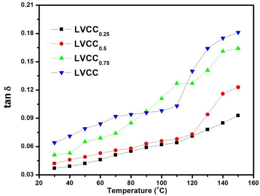
Figure 6: Variation of dielectric loss with temperature at 1kHz for LVCC crystals
