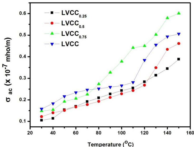
Figure 10: Variation of AC conductivity with temperature at the frequency of 1 kHz for LVCC crystals
