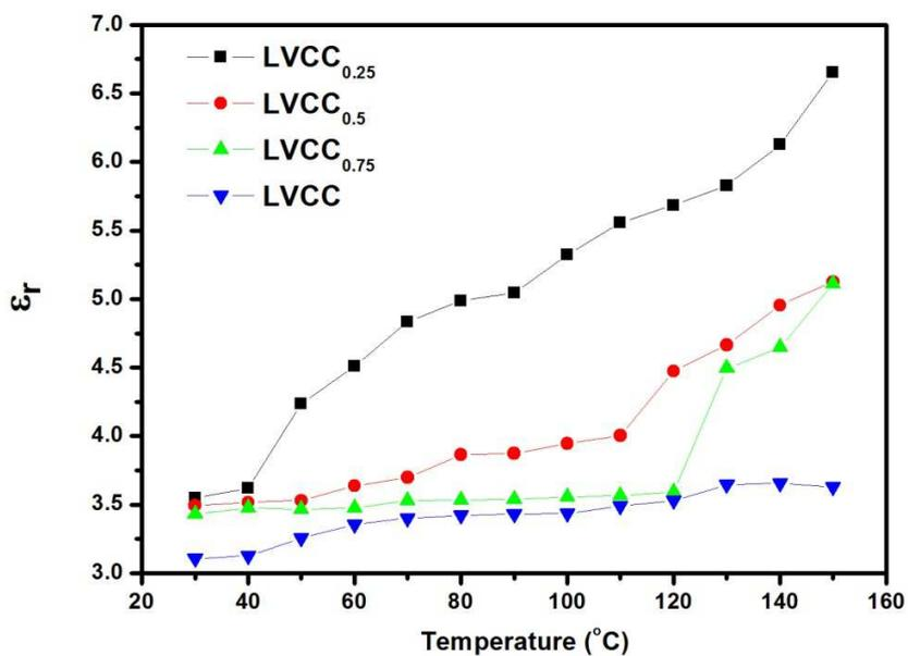
Figure 4: Variation of dielectric constant with temperature for different concentration CdCl<sub>2</sub> mixed LVCC crystals at 100 kHz
