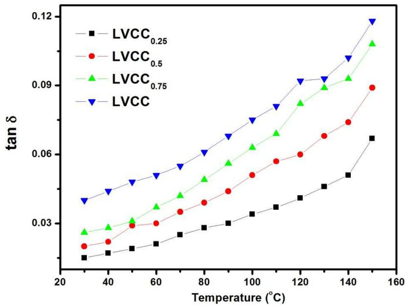
Figure 9: Variation of dielectric loss with temperature at frequency of 1 MHz for LVCC crystals
