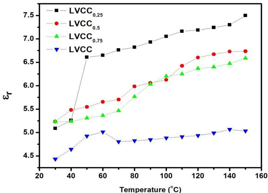
Figure 2: Variation of dielectric constant with temperature for different concentration CdCl<sub>2</sub> mixed LVCC crystals at frequency of 1 kHz
