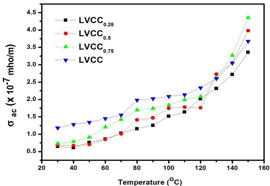
Figure 11: Variation of AC conductivity with temperature at the frequency of 10 kHz for LVCC crystals
