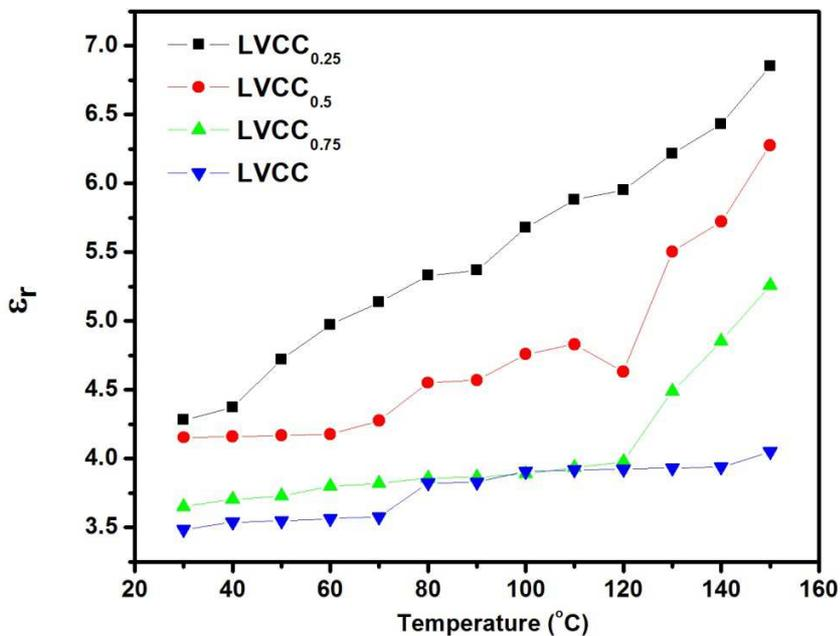
Figure 3: Variation of dielectric constant with temperature for different concentration CdCl<sub>2</sub> mixed LVCC crystals at 10 kHz
