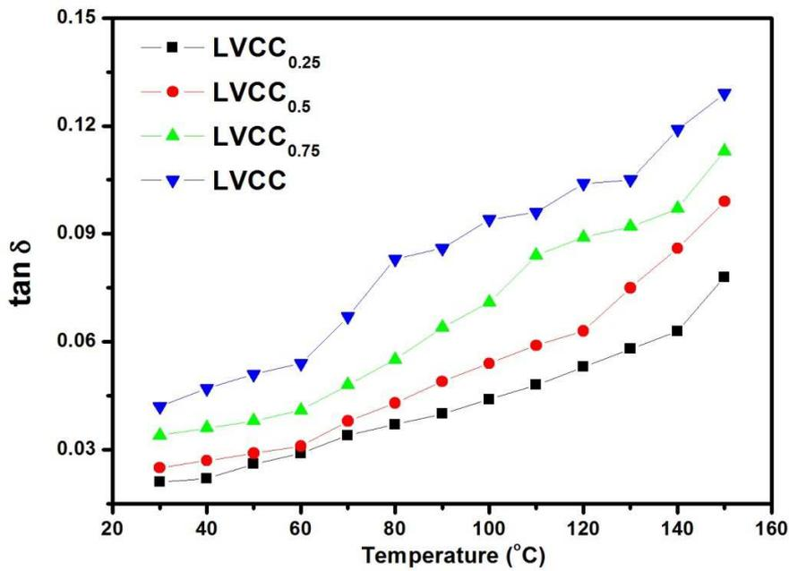
Figure 8: Variation of dielectric loss with temperature at 100 kHz for LVCC crystals
