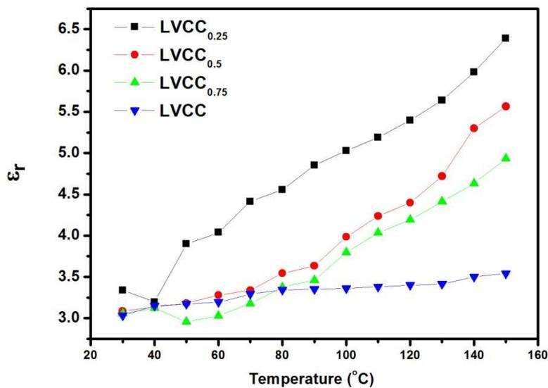
Figure 5: Variation of dielectric constant with temperature for different concentration CdCl<sub>2</sub> mixed LVCC crystals at frequency of 1 MHz
