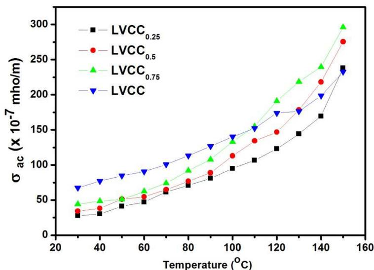
Figure 13: Variation of AC conductivity with temperature at the frequency of 1 MHz for LVCC crystals
