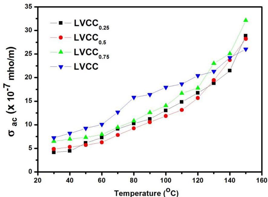
Figure 12: Variation of AC conductivity with temperature at the frequency of 100 kHz for LVCC crystals
